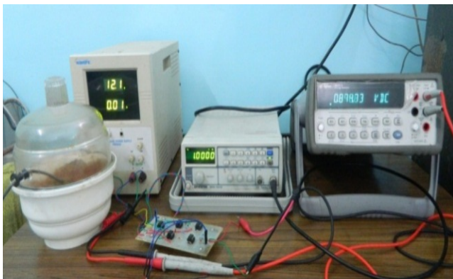
Fig. 6: Laboratory setup for measurement of the soil moisture
